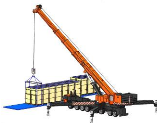
Long-side vertical package unloading with crane
