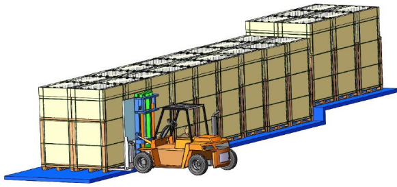
Long-side vertical package unloading with forklift
